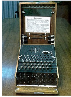
Figure 1.1: Enigma machine, used by the German military sending secret codes during World War II.
