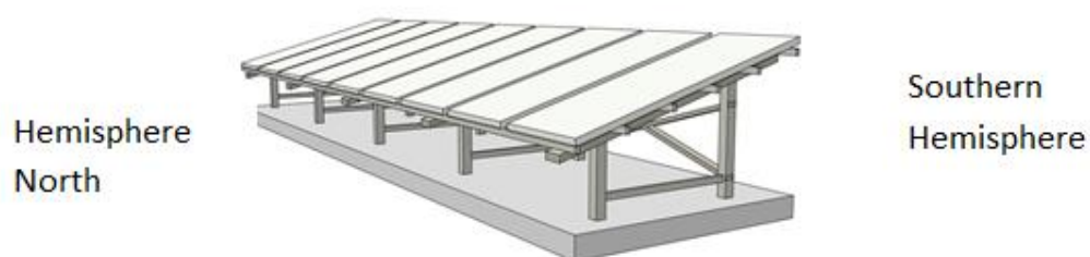
Figure2.2: The direction in which the solar panels are facing at all Burundian sites.
