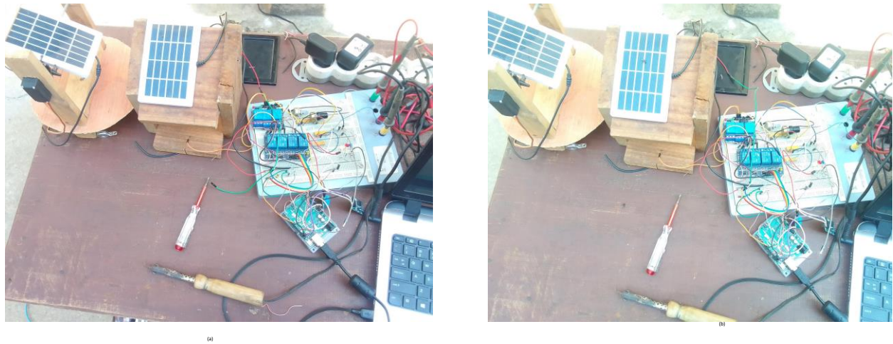
Figure3.56: Experimental assembly of a solar tracker with a battery charging and discharging management system
