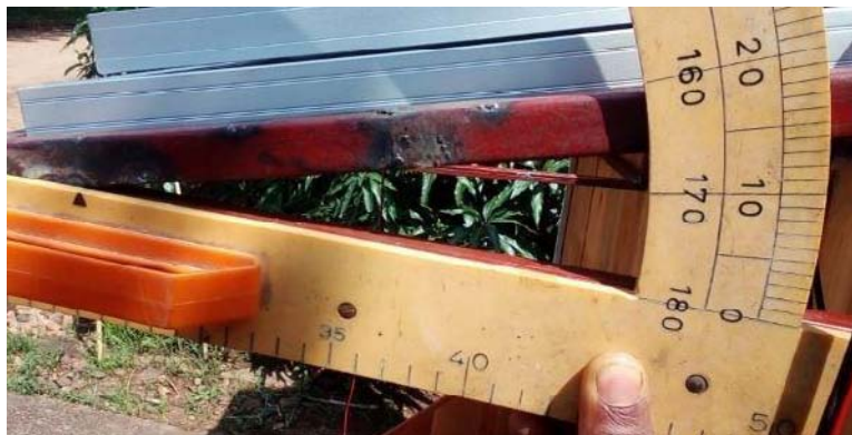
Figure3.9: Photovoltaic solar panel has a 14^\circ slant.
