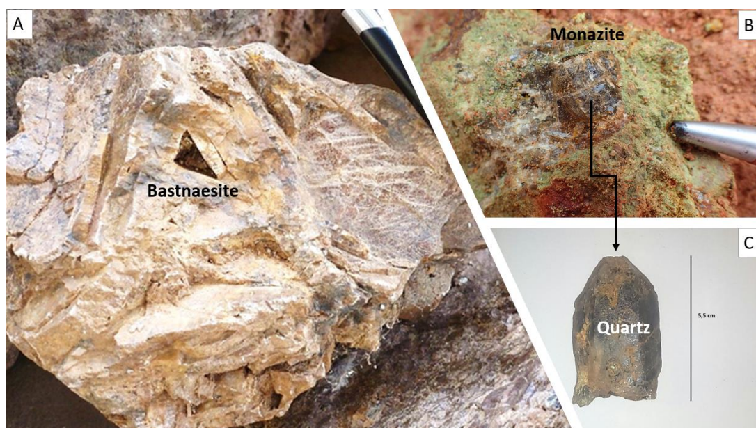
Figure 3: a) Coarse-grained, monomineralic bastnaesite ore; b) Fine-grained, monazite-rich ore associated with large euhedral crystals of dark quartz (c).
