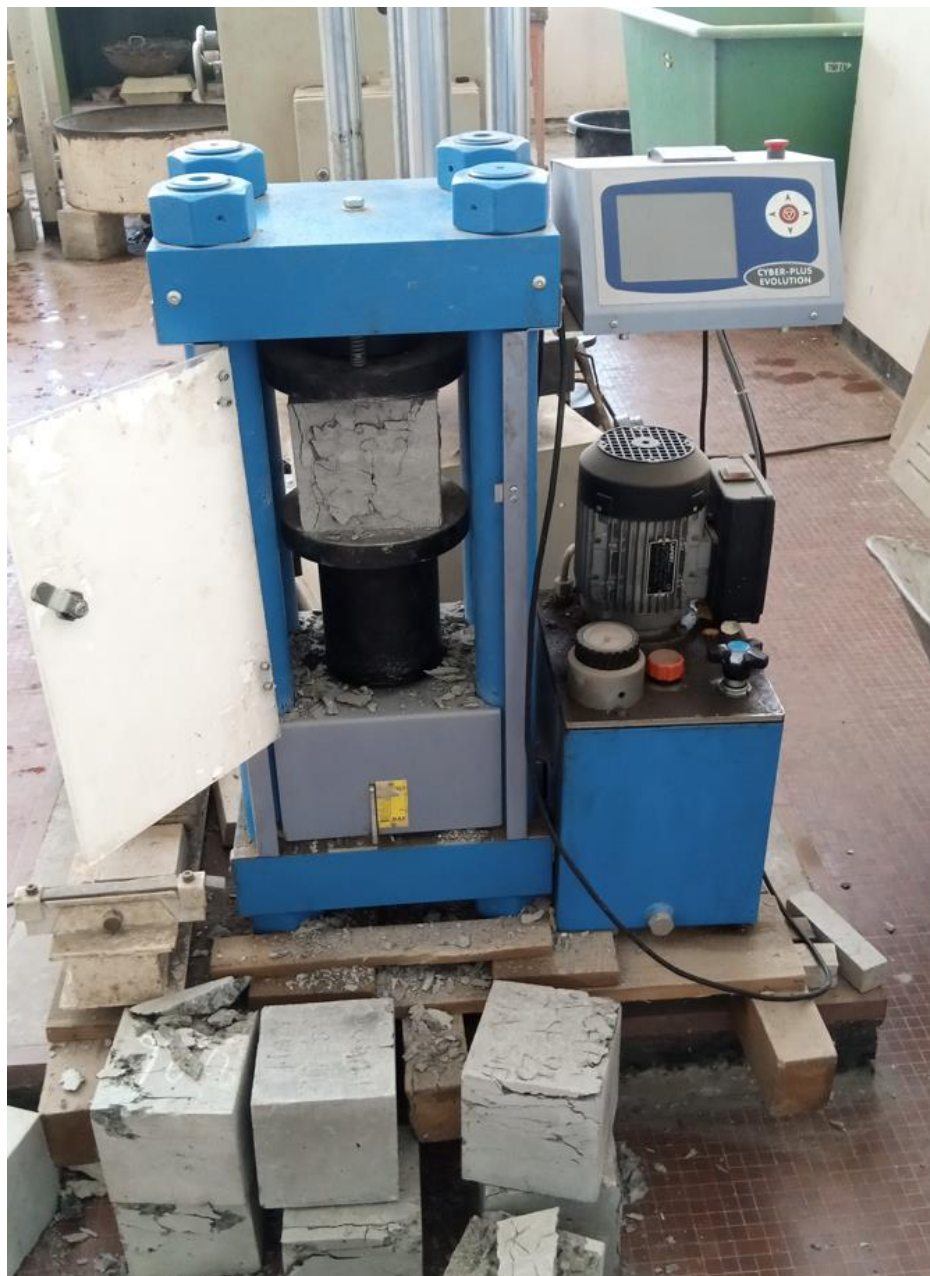
Figure II.15 : Photo illustrant l'essai de compression
